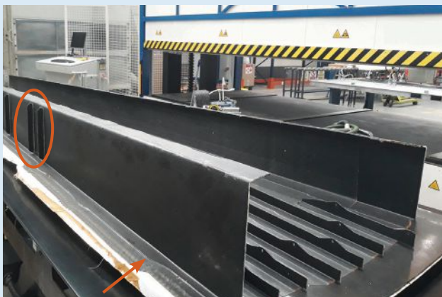
7 Initial demonstrator completed at MTorres shows the J-spacer with two rib stiffeners (circled) and its sinusoidal feet (arrow).
