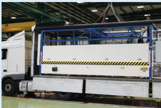
8 ACTI forming/curing equipment and wing box tooling were lifted onto a standard moving truck and relocated to Airbus DS in Cadiz, Spain.
