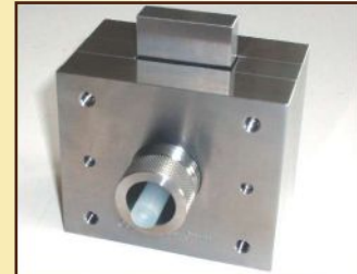
Amsler Double Shear Test Fixture ASTM B 769
