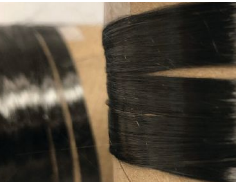
■ 4M large-diameter carbon fiber made with Dralon textile-grade precursor. Source | 4M Carbon Fiber
