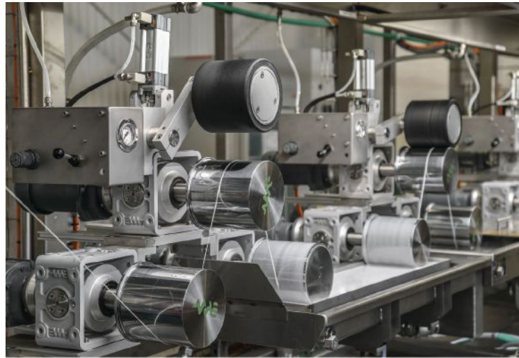
■ CSIRO's wet spinning line, including rollers for controlled stretching.
