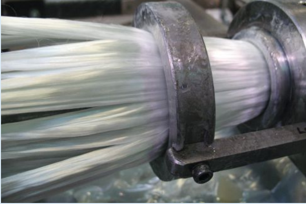
1 Glass fiber is fed into the pultrusion die and injected with resin in a closed-molding process.
