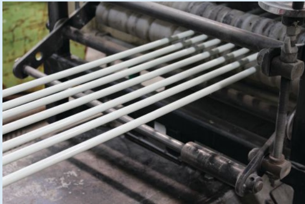
2 The pultrusion process creates glass fiber/vinyl ester composite rods in length of up to 80 feet.
