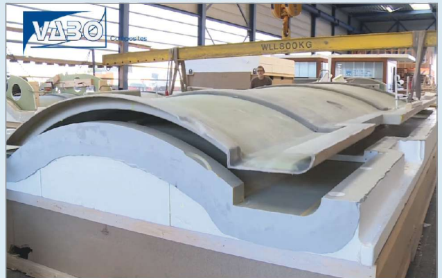
4 Infused glass fiber/vinyl ester parts were demolded.
