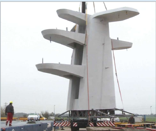
9 A single-piece mast is crane-lifted and prefit to the yacht, followed by final systems installation, exterior painting and, at last, final installation onto the yacht.
