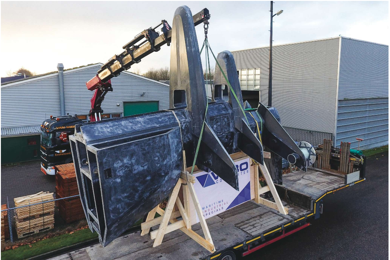
FIG. 3 Vabo Composites' second mast project will install this carbon fiber/epoxy radar mast on top of the canopy shown on p. 33 to form a single-piece, installation-ready assembly for a 90m-long yacht.
