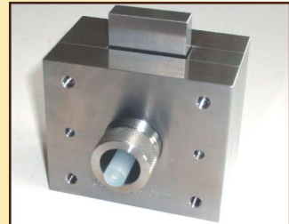
Amsler Double Shear Test Fixture ASTM B 769
