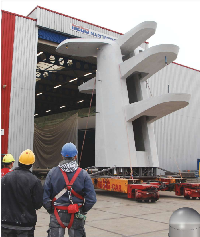
FIG. 1 The 10-by-10-by-10m glass fiber/vinyl ester mast for a 156m-long yacht (left) features two legs joined to form a “T” from which four platforms extend, three forward and one rearward.
