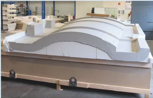
1 Vabo Composites CNC-machined 10 molds for the glass fiber/vinyl ester mast project (shown here) and seven molds for the carbon fiber/epoxy project comprising mast and canopy.
