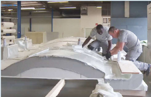
2 Parts fabrication began with laying glass reinforcements onto molds, along with perforated foam core, to create a dry laminate stack.
