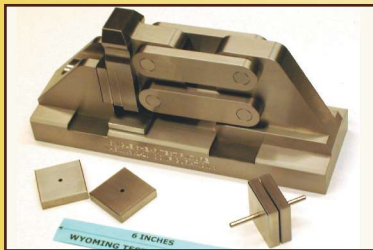
Fastener Single Shear Test Fixture NASM 1312-20
