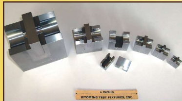
Fastener Double Shear Test Fixtures NASM 1312-13
