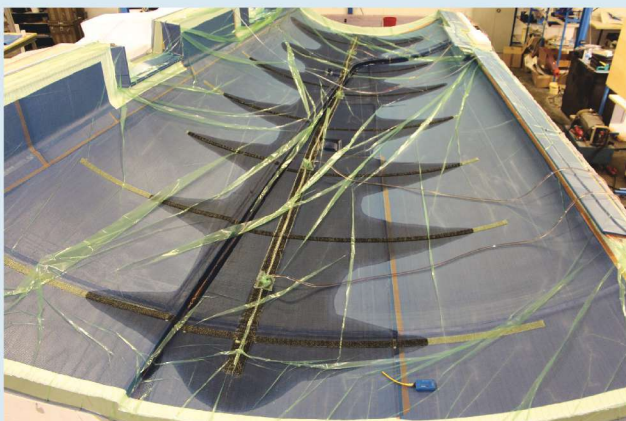
3 Dry stacks were vacuum bagged and Vabo Composites' one-shot resin infusion method was employed for the glass fiber/vinyl ester mast, with legs and platforms completed in 2-3 hours.
