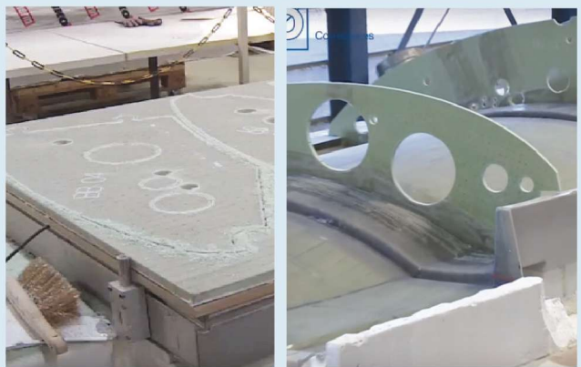
5 Reinforcing ribs were CNC machined — including holes for cables and exhaust pipes — from resin-infused, foam-cored glass fiber/vinyl ester flat panels (left image). Ribs were then bonded to the mast legs at roughly 1m intervals (right image).
