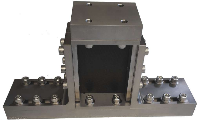
FIG. 3b Compression-after-impact test, ASTM D 7137.
