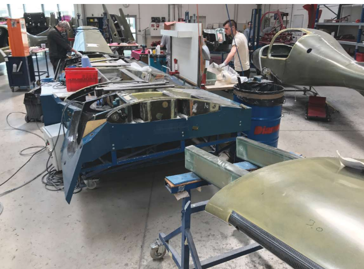
FIG. 7 Pre-fit, postcure, paint and final assembly
