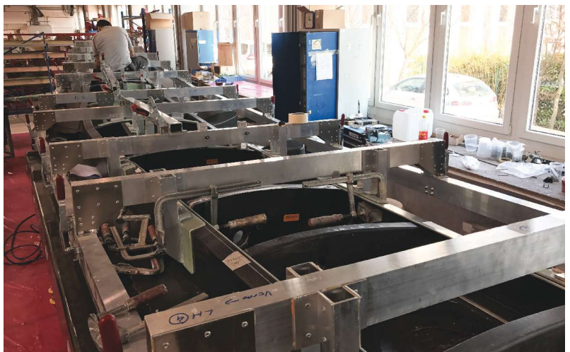
FIG. 4 Interchangeable bonded wing structures
