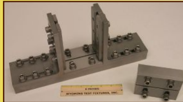
Boeing Compression After Impact ASTM D 7137
