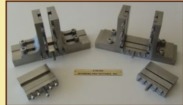
Airbus Compression After Impact AITMI - 0010
