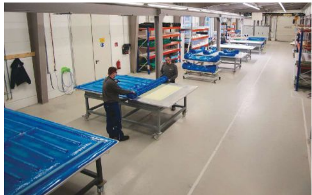
FIG. 2 Light RTM rail floors
