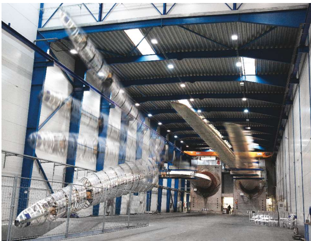
FIG. 7 Static and fatigue testing
