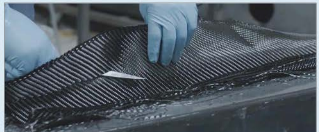
2 Solvay MTM45-1 prepreg fabric is precision cut by automated ply cutter or hand cut by skilled technicians. Gerbercutter from Gerber Technology (Tolland, CT) performs automated ply cutting (top); a TSC technician hand-cuts prepreg to small shapes for custom layup (bottom).
