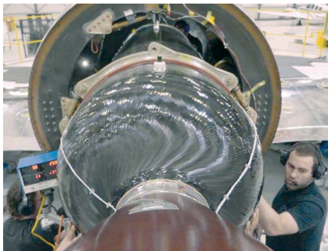
FIG. 3 Composite parts for engine installation
