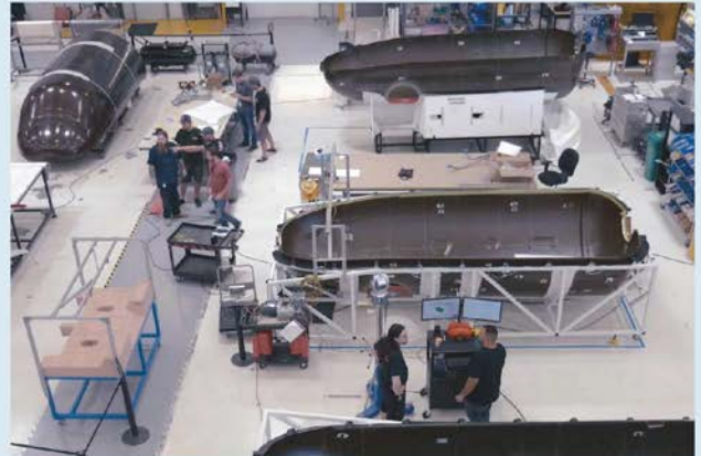
1 Tooling is prepared for carbon fiber composite layup of new SpaceShip fuselage sections SS2-003 and SS2-004 . Tooling preparations include waxing, and application of an appropriate mold release and primer.
