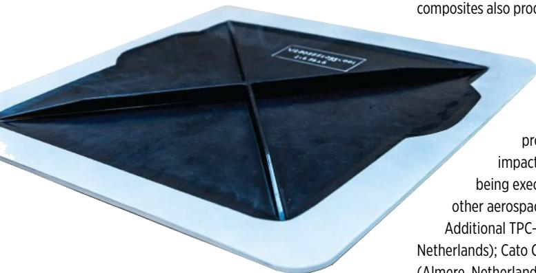
■ A demonstrator of the recycled carbon fiber/PPS access door panel. Source | TPAC
