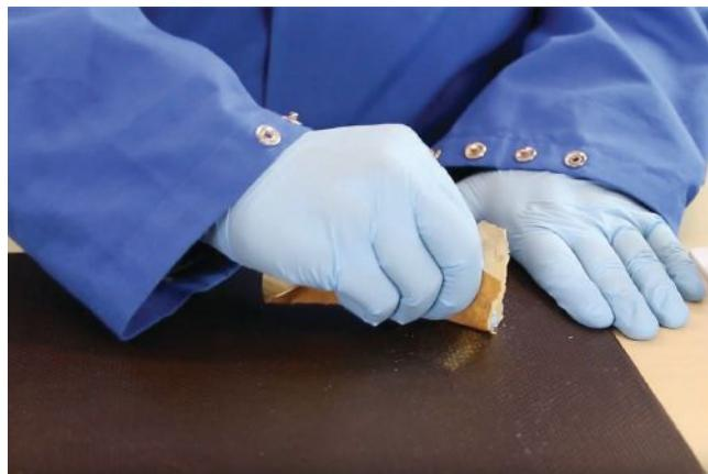
■ Manual abrasion is a common method of surface preparation for composites, but it may not be effective at cleaning a surface on its own.
