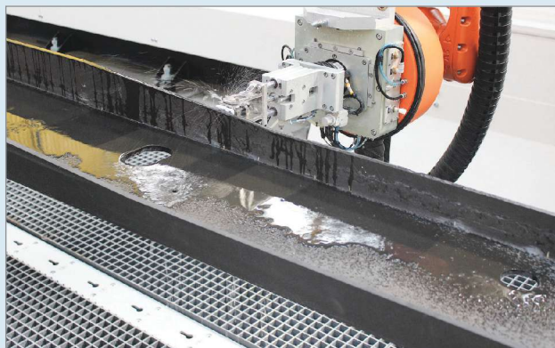
7 A cured spar undergoes ultrasonic nondestructive inspection. After inspection, the front and rear spar, the metallic ribs and the skins/stringers are assembled with mechanical fasteners.
