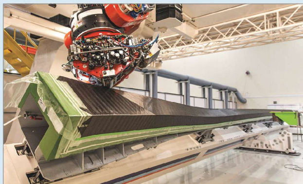
6 The front and rear spars of the MS-21 wing are laid up in one piece on a male mold using an MTorres system. Solvay says the PRISM TX 1100 material has proven uncommonly steerable, which means it can accommodate varying angular placement with no wrinkling. Thus, AeroComposit has avoided the more conventional practice of building spars that require angular displacements in separate sections that must be secondarily bonded/fastened.
