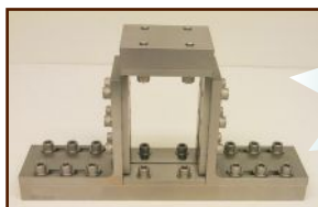
Boeing Compression After Impact Test Fixture ASTM D 7137
