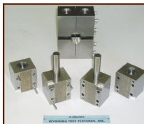
Combined Loading Compression Test Fixture ASTM D 6641
