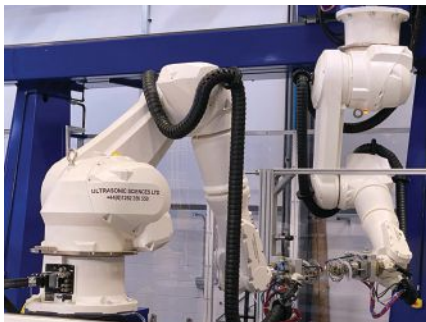
Ultrasonic NDI is conducted by two robots working in unison.
