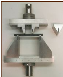
Three & Four Point Flexure Test Fixture ASTM D 790, 6272, 7264
