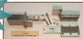
Boeing Open-Hole Compression Test Fixture ASTM D 6484
