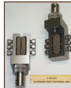
V-Notched Rail Shear Test Fixture ASTM D 7078
