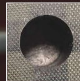
Hole drilled with Allied's T-A PCD tooling
