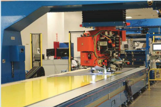
1 Material is prepared for Automated Spar Forming on a Material Preparation Machine, which unrolls, collates, re-ori-ents and re-rolls prepreg.
