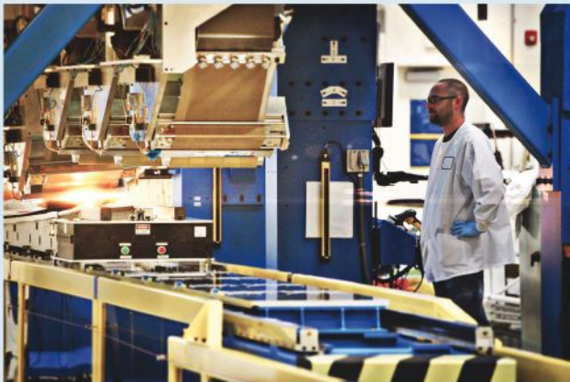
2 As it lays down material, the linear Automated Spar Forming Machine (ASFM) passes a series of rollers and forming devices over the material, simultaneously compacting and debulking it tightly against the tool and underlying laminate, so that separate debulk cycles are not required.
