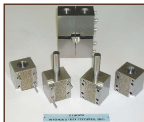
Combined Loading Compression Test Fixture ASTM D 6641
