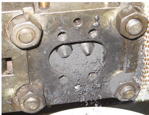
Fraunhofer ICT's ReUse project uses reaction processing to devulcanise EPDM. Images show the vulcanised material at the extruder exit (left) and final raw polymer (right)
