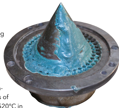
Above and left: Before and after images showing a pelletising plate that has been cleaned at Schwing Image: Schwing Technologies
