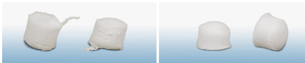
Coperion's new EGR knife minimises fine generation. Pellets produced on the new system (right) shown compared to current technology
