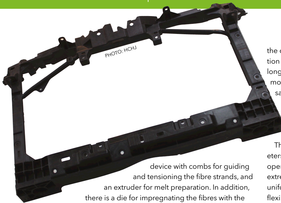
Above: An automotive front-end module produced in LFT-PP
