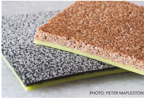
Right: Samples cut from rotomouldings showing the unusual finish of Beologic compounds containing denim fibres (left) and cork
