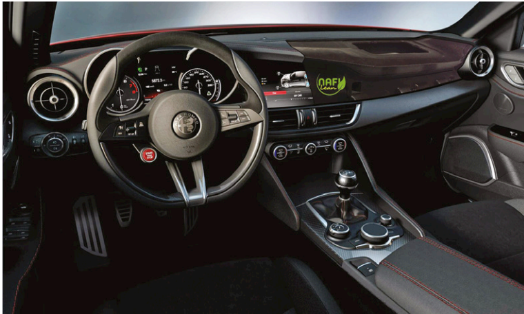
Above: NAFIlean, from Faurecia and Interval JV APM, is used in the instrument panel of Alfa Romeo's flagship saloon, the Giulia
