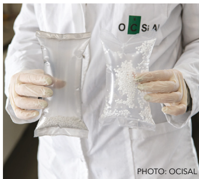
SWCNTs reduce static in the new PE film (left)
