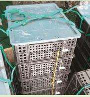
Antimicrobial technology from Parx Materials eliminated fouling on plastic tanks used to farm abalone shellfish. These images show the results after six months in the sea (both were new at the outset)
