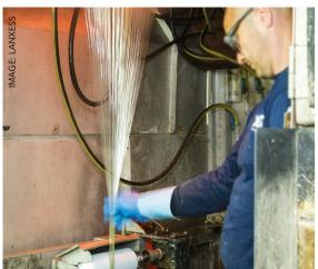
Glass fibre production at the Lanxess plant at Antwerp
