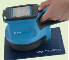
of a wide variety of plastic or painted surfaces, ranging from leather-like to fine-textured and smooth. It features an icon-based colour touchscreen control while an integrated camera shows a live preview of the measurement spot to prevent false readings on imperfections or scratches.
