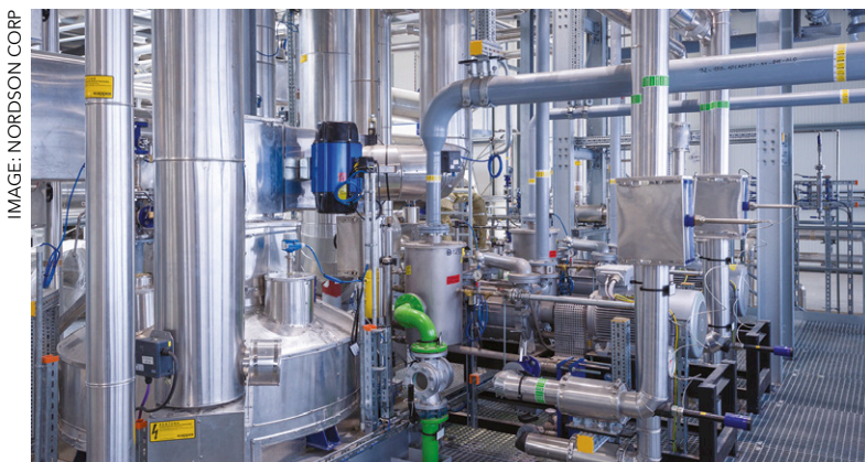
Above: APK's Newcycling plant at Mereseburg in Germany recycles multi-layer post-industrial film using Nordson BKG pelletising technology
