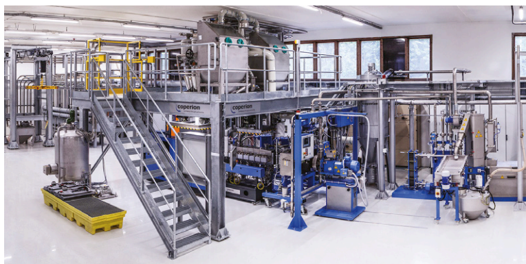
Above: This turnkey compounding line was supplied to Finnish conductive polymer producer IonPhasE. It uses an underwater pelletiser supplied by Nordson BKG
