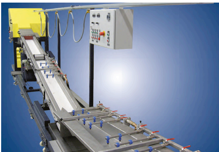
Right: ips Intelligent Pelletizing Solutions now has an ips-SGA 220/2 automatic strand pelletising system available for internal development and customer trials at its German technical centre
