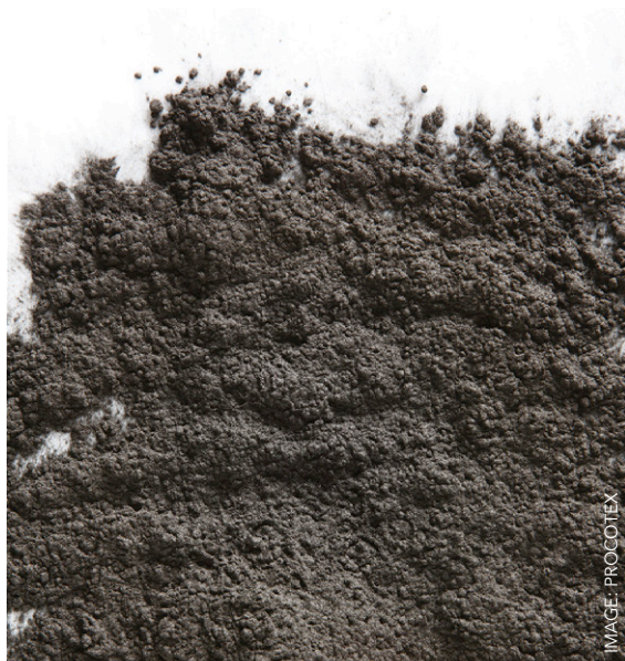
Right: Milled carbon fibre produced by Procotex from composite waste
