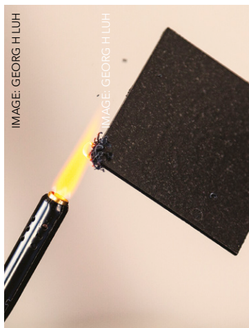
Above: A flame being put to a PA compound filled with expandable graphite
