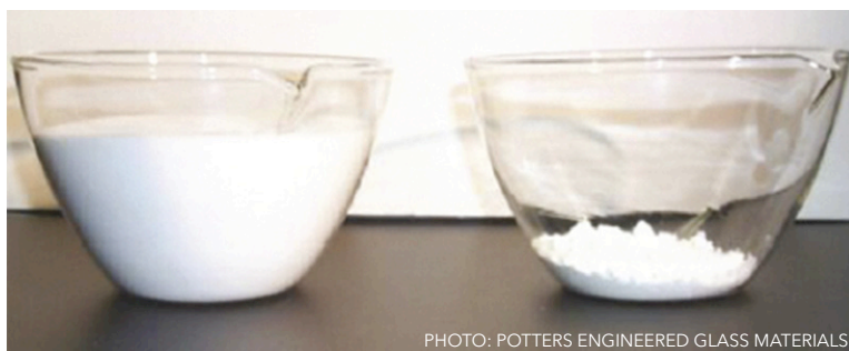
Above: Equal weights of hollow glass microspheres (left) and mineral filler (right) showing the potential density reduction
