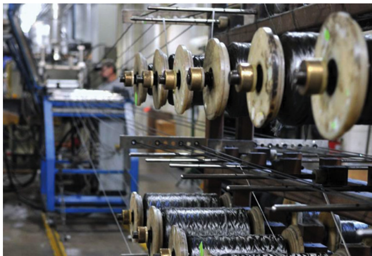
Above: Stainless steel fibres go into electrically conductive long fibre filled compounds at RTP Company
