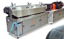
ENTEK manufactures co-rotating twin-screw extruders in sizes ranging from 27mm to 133mm.
