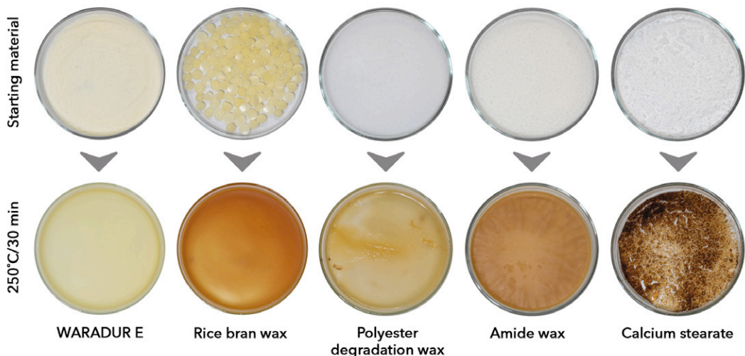
Figure 2: Colour stability under stress of Waradur E hard ester montan wax compared to some current alternatives (Heraeus UT 6120 laboratory air circulation oven; 250°C/ 30 min)
